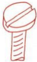
Screwdriver can slip and scratch surface
