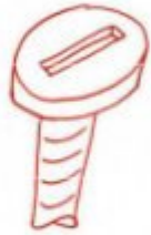
Screwdriver can't slip and scratch surface
